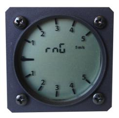
Here you can then select vario Range between 2.5m/s, 5m/s and 10m/s, or 5kts, 10kts and 20kts.
